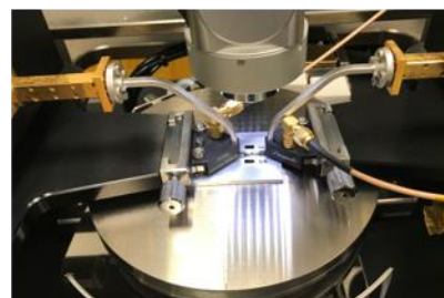
RF on-wafer measurement (750 GHz in ambient, 40 GHz cryogenic)
